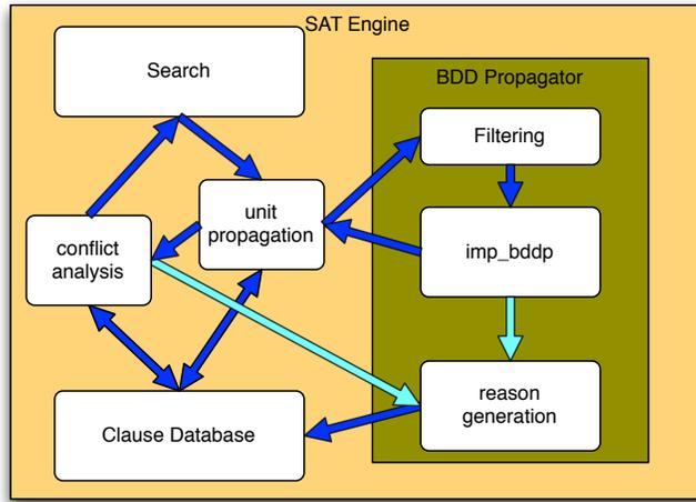
Figure 14: Architecture for the hybrid BDD-SAT solver.
