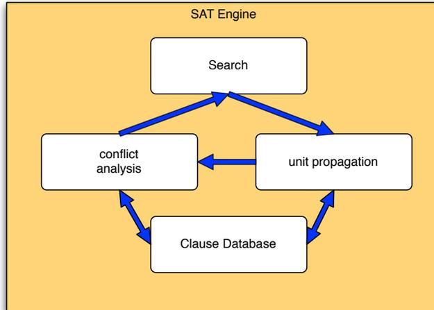
Figure 1: Architecture for the SAT solver.
