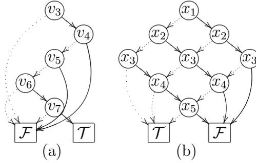
Figure 2: BDDs for (a)  $v_3 \wedge \neg v_4 \wedge \neg v_5 \wedge v_6 \wedge v_7$ . (b)  $x_1 + x_2 + x_3 + x_4 + x_5 \leq 2$ . The node  $n(v, f, t)$  is shown as a circle labelled  $v$  with a dotted arc to the  $f$  BDD, and a solid arc to the  $t$  BDD.
