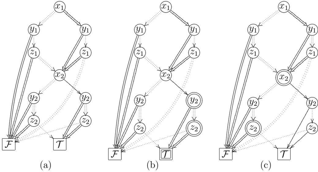
Figure 13: (a) The BDD representing  $x = y \cup z$  where  $N = 2$ , with  $E[y_1] = \{1\}$ ,  $E[z_2] = \{1\}$  and  $E[x_2] = \{0\}$ . Edges consistent with the partial assignment are shown doubled. (b) Nodes which must remain unreachable in the reason are shown doubled. (c) Edges reachable along the minimal reason are shown doubled, as are nodes which remain fixed.
