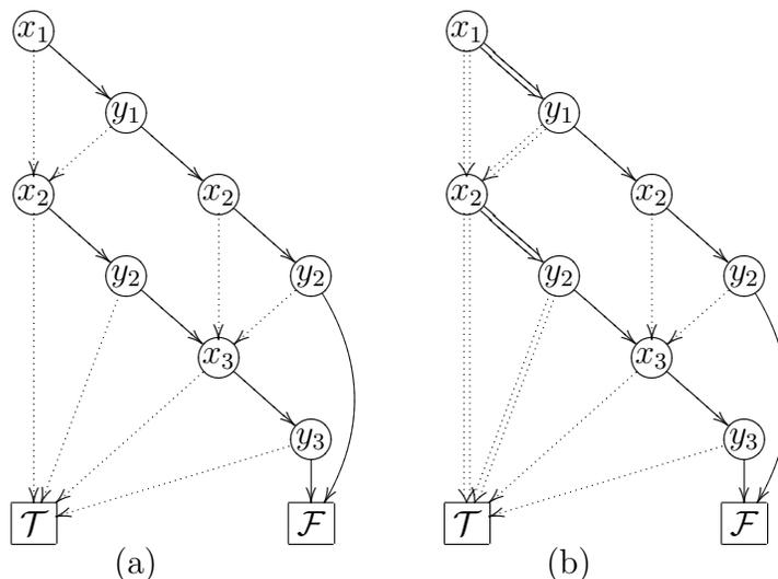
Figure 11: (a) The BDD representing  $|x \cap y| \leq 1$  where  $N = 3$ . A node  $n(v, f, t)$  is shown as a circle around  $v$  with a dotted arrow to  $f$  and full arrow to  $t$ . (b) The edges traversed by `imp_bddp`, when  $E[v] = \{0, 1\}$  for all  $v$ , are shown doubled.
