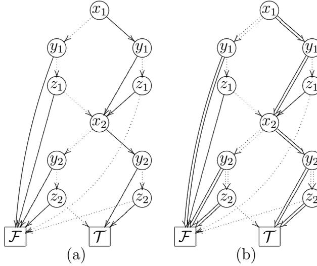
Figure 6: (a) The BDD representing  $x = y \cup z$  where  $N = 2$ . (b) The edges traversed by `bddprop`, when  $E[y_1] = \{1\}$  and  $E[z_2] = \{1\}$  and  $E[v] = \{0, 1\}$  otherwise, are shown doubled.
