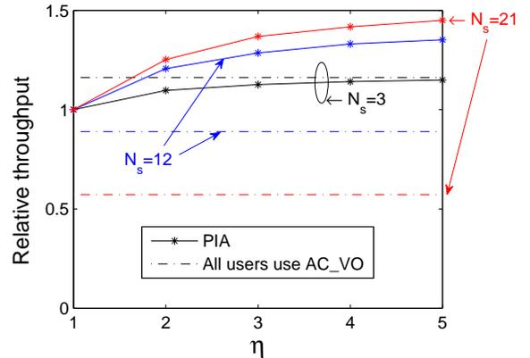
Fig. 5. Throughput of a data user under PIA as a function of class  $B_2$ 's TXOP limit in units of  $\mathcal{T}(\eta)$ , scaled by that of PIA at  $\eta = 1$ . PIA gives better throughput than the default setting with data users using AC\_VO class, except at light load. ( $\lambda = 35$  packets/s,  $l_{\text{sat}} = 1000$  bytes,  $l_{\text{nonsat}} = 200$  bytes,  $N_u = 6$ ,  $W_{B_1} = 32$ ,  $W_{B_2} = \eta W_{B_1} - \epsilon^0$  for  $\eta = \{1, 2, 3, 4, 5\}$ .)
