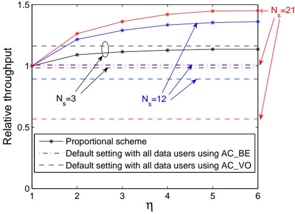
(a) Data throughput. Proportional allocation gives higher throughput than the default setting with data users using AC\_BE class. For heavy load, it also gives better throughput than the default with data users using AC\_VO.
