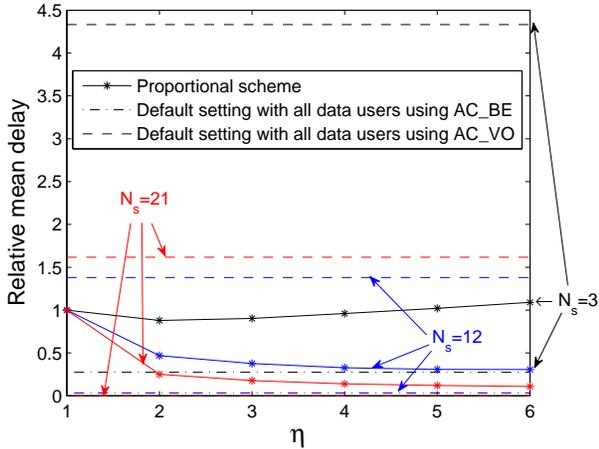
(b) Real-time delay. Proportional allocation gives lower delay than the default setting with data users using AC\_VO, though higher delay than the default with data users using AC\_BE.
