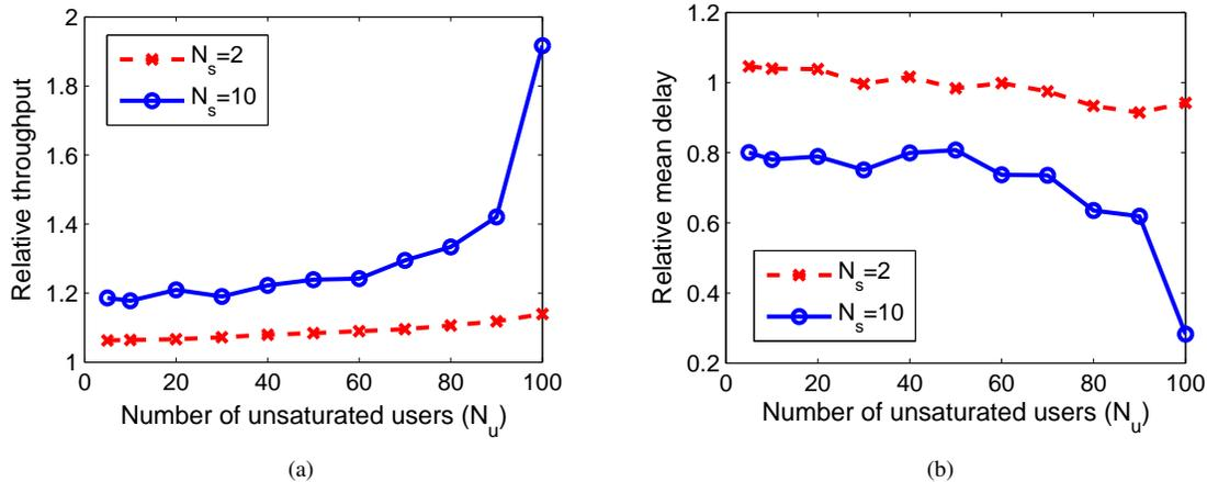
Fig. 9. Ratio of throughput of a data user under PIA at  $\eta = 2$  to that under no service differentiation ( $\eta = 1$ ) and the corresponding ratio of mean delay of a real-time user as a function of the number of realtime users. ( $\lambda = 9$  packets/s,  $l_{sat} = 1200$  bytes,  $l_{nonsat} = 100$  bytes,  $\eta = 2$ ,  $W_{B_1} = 32$ ,  $W_{B_2} = \eta W_{B_1}$ .)
