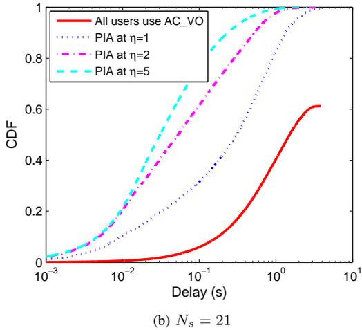
Fig. 6. Probability a packet of real-time users is successfully delivered as a function of delay. ( $\lambda = 35$  pkts/s,  $l_{sat} = 1000B$ ,  $l_{non-sat} = 200B$ ,  $N_u = 6$ ,  $W_{B_1} = 32$ ,  $W_{B_2} = \eta W_{B_1} - \epsilon^0$  for  $\eta = \{1, 2, 5\}$ .)
