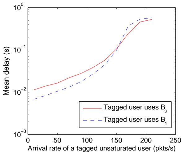
Fig. 10. Mean delay of of the tagged “unsaturated user” as a function of its arrival rate. ( $\lambda_{u \neq 1} = 40$  pkts/s,  $l_{sat} = 1200$ B,  $l_{nonsat} = 100$ B,  $N_u = 10$ ,  $N_s = 5$ ,  $W_{B_1} = 32$ ,  $W_{B_2} = \eta W_{B_1} - \epsilon^0$ ,  $\eta = 2$ .)
