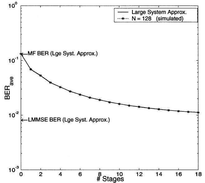
Fig. 4. BER versus stages ( $\alpha = 0.75$  and SNR = 12 dB).
