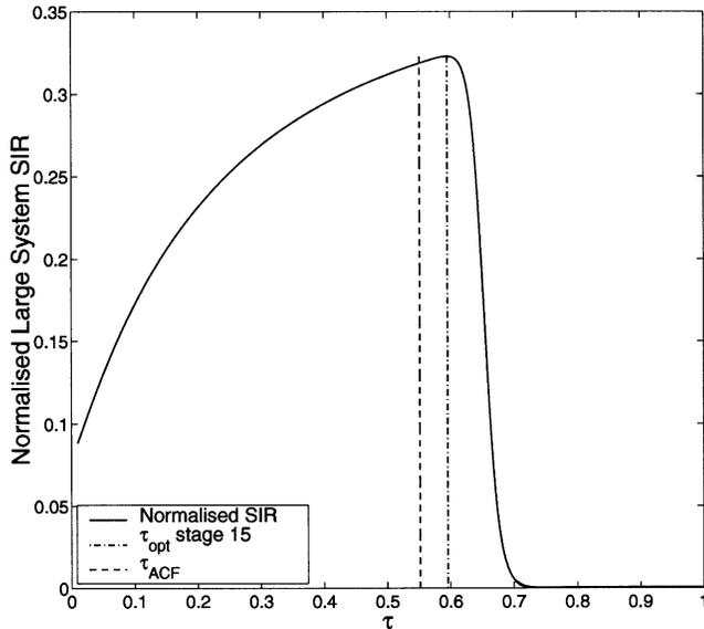
Fig. 2. Large system SINR versus  $\tau$  ( $\alpha = 0.75$ ,  $m = 15$ , and SNR = 12 dB).
