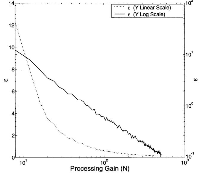
Fig. 1. Empirical MSE versus  $N$  ( $8 \leq N \leq 512$ ,  $\alpha = 0.75$ , and  $\text{SNR} = 12$  dB).
