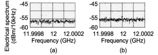
Fig. 3. RF spectra of the signal and beat noise after (a) one photodiode and (b) balanced subtraction, OSNR = 16 dB, PRBS pattern length =  $2^{31} - 1$ , with RF amplifier ON.
