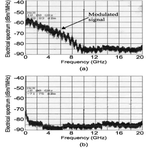
Fig. 2. RF spectra of the signal after (a) one photodiode and (b) balanced subtraction, with ASE source turned OFF and RF amplifier bypassed.
