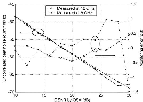
Fig. 4. Measured uncorrelated beat noise power density and the monitoring error versus the OSNR measured by the OSA.
