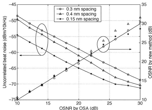
Fig. 5. Comparison of the measured uncorrelated beat noise power density and the measured OSNR by the proposed method at different spacings of the filters versus the OSNR measured by the OSA.
