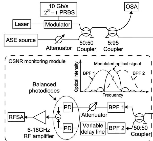
Fig. 1. Experimental setup. (BPF: Bandpass filter. PD: Photodiode.)
