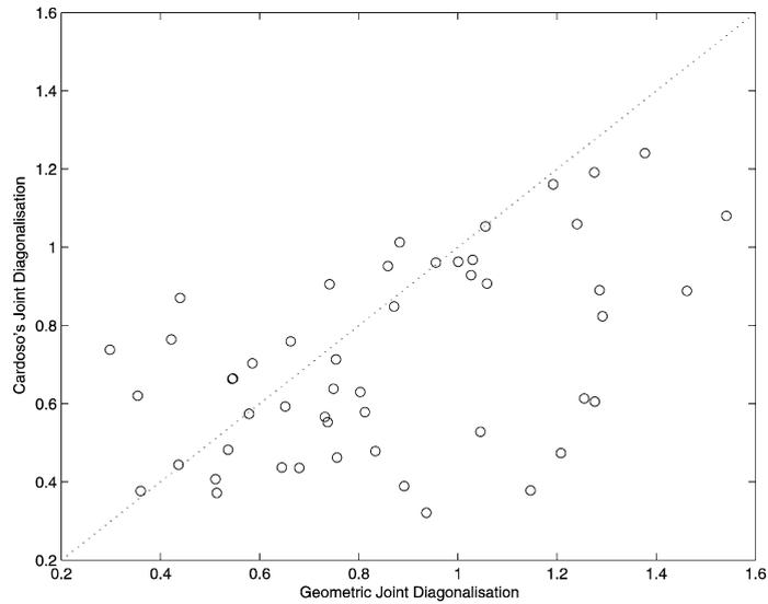
Fig. 4. For noise model one, Cardoso's method has a mean error of 0.71 and a standard deviation of 0.25 while the geometric joint diagonaliser has a mean error of 0.86 and a standard deviation of 0.32.
