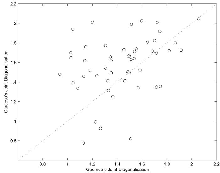
Fig. 5. For noise model two, Cardoso's method has a mean error of 1.58 and a standard deviation of 0.30 while the geometric joint diagonaliser has a mean error of 1.43 and a standard deviation of 0.26.
