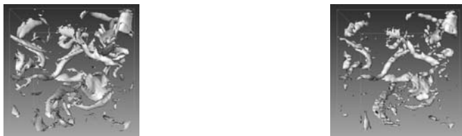
Figure 2: Isosurfaces of enstrophy of (a) the original unfiltered vorticity field and (b) Filtered (at \epsilon = \epsilon_d ) vorticity field.
