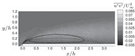
Figure 5: Reynolds shear stress contours  $\overline{u'v'}/U_\infty^2$ ;  $\delta/h = 1.35$ ;  $Re_h = 6741$
