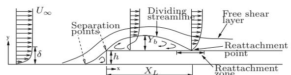
Figure 1: Flow features over a forward facing step
