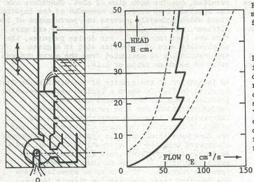
Fig 1 (left) illustrates the use of a vortex modulator to produce a nearly constant discharge from a storage reservoir. (Brombach)
