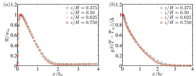
Figure 3: Mean profiles of (a) Vertical velocity and (b) buoyancy at  $0.375 \leq z/H \leq 0.75$  for the  $R/H = 2$  case.
