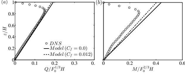
Figure 4: Comparison of mean (a) volume and (b) momentum flux with the theoretical model in a uniform environment. The black circle represents the DNS results, the black solid and dashed lines represent the theoretical model with  $c_f = 0.0$  and  $c_f = 0.012$ , respectively.
