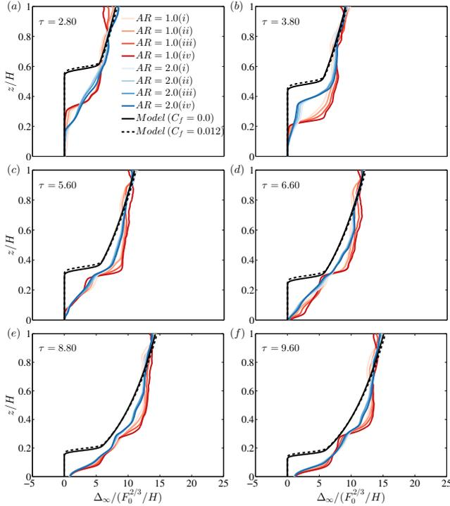
Figure 5: Comparison of the time-dependent environmental buoyancy profile with theoretical model for  $AR = 1.0$  and  $AR = 2.0$ ; (a)  $\tau = 2.80$ ; (b)  $\tau = 3.8$ ; (c)  $\tau = 5.6$ ; (d)  $\tau = 6.60$ ; (e)  $\tau = 8.8$ ; and (f)  $\tau = 9.6$ . The colour gradients of red and blue indicate the starting point of horizontal average for two different aspect ratios; (i) for horizontal average from  $x/H = 0.2$ , (ii) for  $x/H = 0.4$ , (iii) for  $x/H = 0.6$  and (iv) for  $x/H = 0.8$ .
