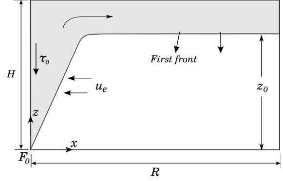
Figure 2: Schematic diagram of filling box model of wall attached line plume. The first front is the interface between buoyant fluid and the ambient fluid. The time-dependant position of the first front position is denoted by  $z_0$ .
