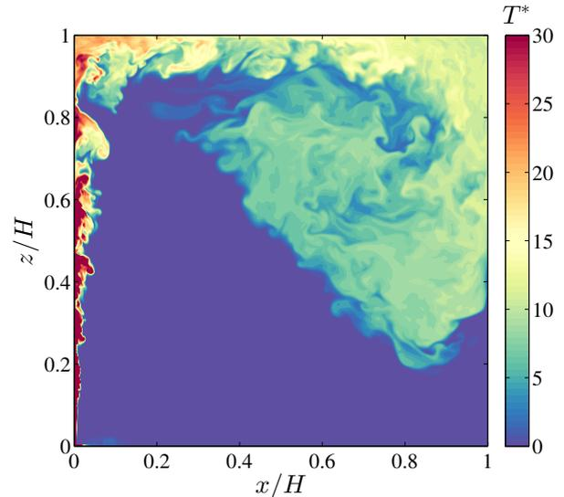
Figure 1: Contour plot of the instantaneous non-dimensional temperature ( $T^*$ ) at  $y/H = 0.5$  for aspect ratio ( $AR$ ) = 1.0.
