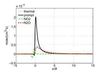
Figure 1. Different pathways of NO formation for the 1D laminar flame
