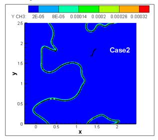
Figure 5. Contours of  $CH_3$  mass fraction in the low turbulence intensity case (case2) – the black line is representing the isoline for T = 1400 K
