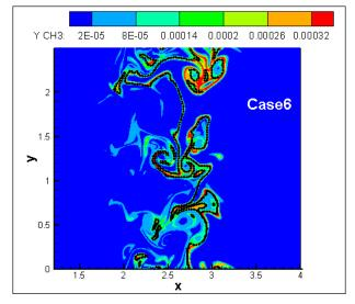
Figure 6. Contours of  $CH_3$  mass fraction in the high turbulence intensity case (case6) – the black line is representing the isoline for T = 1400 K
