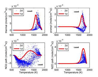
Figure 3. NO pathways for the high turbulence intensity case (case6)
