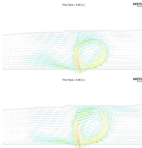
Figure 5. Instantaneous vector fields near the printhead. Paper motion is from right-to-left.
