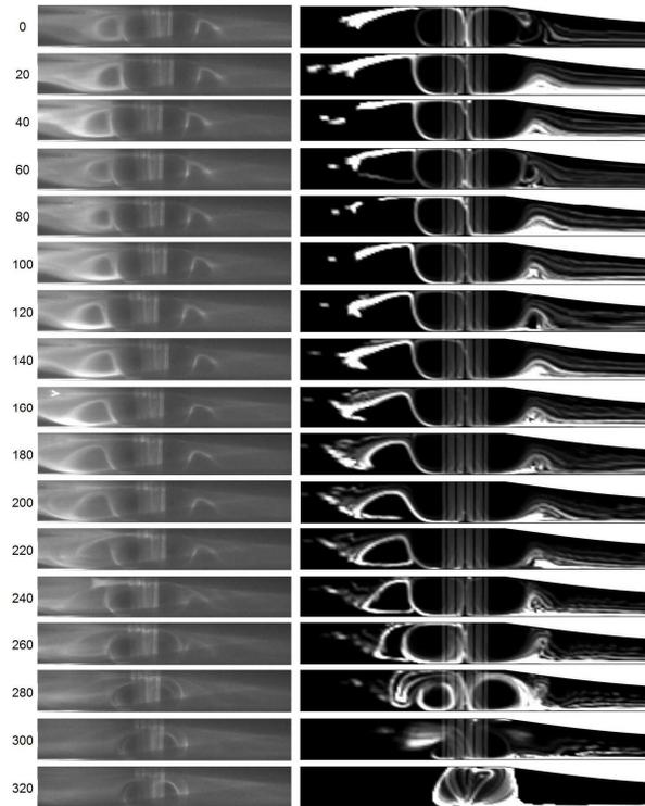
Figure 4. Comparison of experimental (left) and numerical (right) droplet concentration. The numbers at the left refer to the number of actuators from the centre of the printing region. Flow is from left-to-right.
