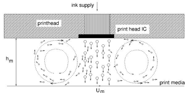
Figure 2. Schematic of the print-zone (not to scale), wherein the printhead IC (PHIC) ejects droplets from several locations onto media located  $h_m$  away from the PHIC and which moves at a speed  $U_m$ . The flow induced by the large droplets causes counter-rotating vortices to be situated either side of the PHIC; these vortices trap smaller particles which can then be re-deposited.
