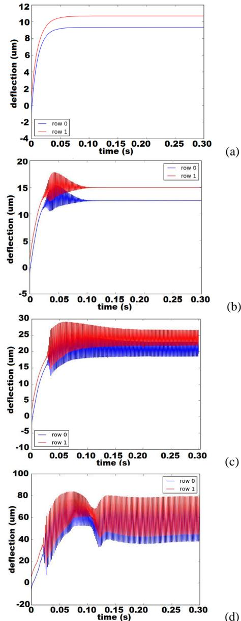
Figure 6. Deflection of main droplets as a function of time for two rows of a single colour plane. (a)  $h_m = 1$  mm; (b)  $h_m = 1.7$  mm; (c)  $h_m = 2$  mm; (d)  $h_m = 3$  mm.
