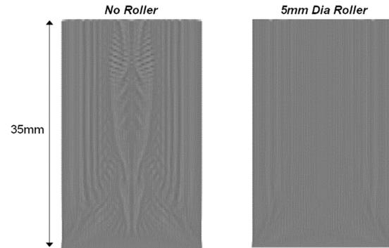
Figure 10. Comparison of numerical prints with and without roller.
