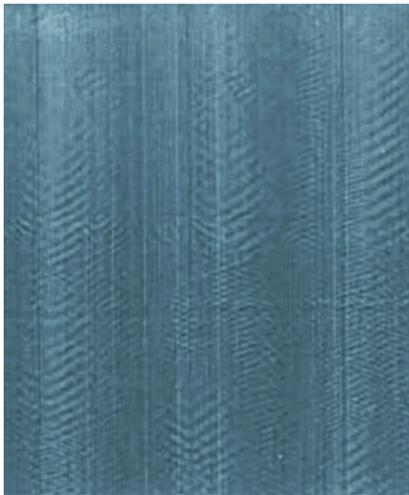
Figure 1. Print sample showing 'tiger striping'.
