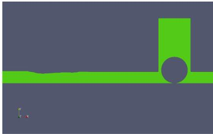
Figure 8. Print-zone with upstream roller, paper moving right-to-left.
