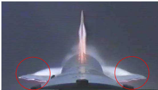
Figure 1. Cameras onboard the SHEFEX-I flight experiment captured the structural deformation of the fins due to severe aerothermodynamic loading during re-entry [1].
