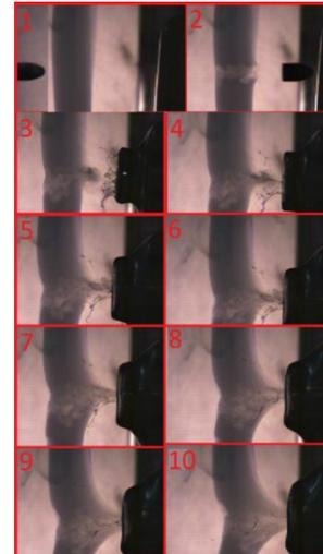
Figure 8. Example of the air motion into 10 % gelatine.
