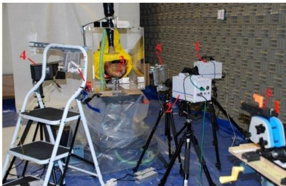
Figure 2. Experimental set up; 1- SA5 2- SA1 3- Sample holder 4- Kaiser Video lamp 5- LED lights 6- Gun
