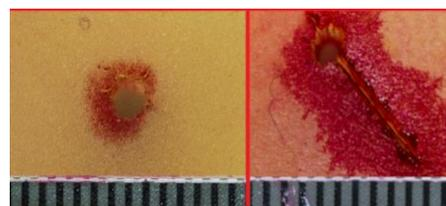
Figure 4. Form of the damage in 10% gelatine with the rigid boundary at right and without boundary at left
