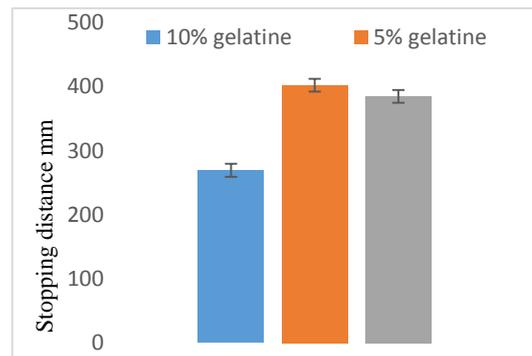
Figure 3. Stopping distance of the projectile in different materials
