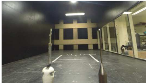
Figure 5. The hot-element anemometer (left) and multi-hole Cobra probe (right) in turbulent flow in the IWT (6m downstream from grid).
