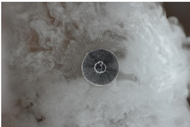
Figure 3. Photograph taken from below the glass base showing cavitation occurrence around the inlet nozzle periphery and the generated microbubble plume from nozzle 3 for K = 0.13 and h/d = 0.08 .
