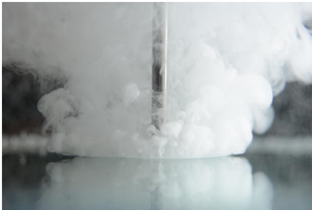
Figure 2. Side photograph of the generated microbubble plume from nozzle 3 for K = 0.13 and h/d = 0.08 .
