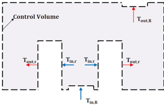
Figure 2. Control volume taken inside the room excluding server racks.
