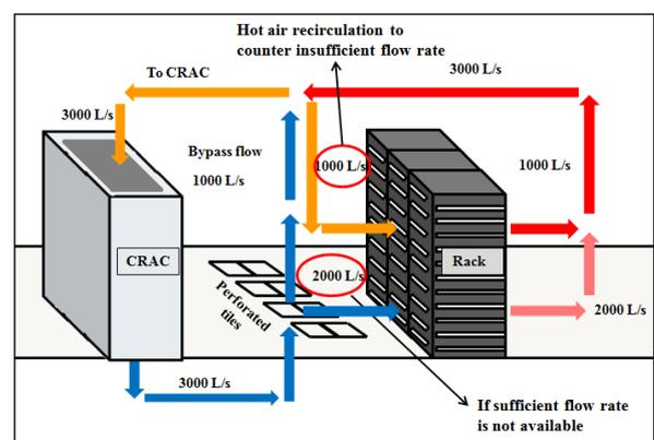
Figure 1. A typical data centre with hot air recirculation and cold air short-circuiting ( total cold air supply of 3000 l/sec).
