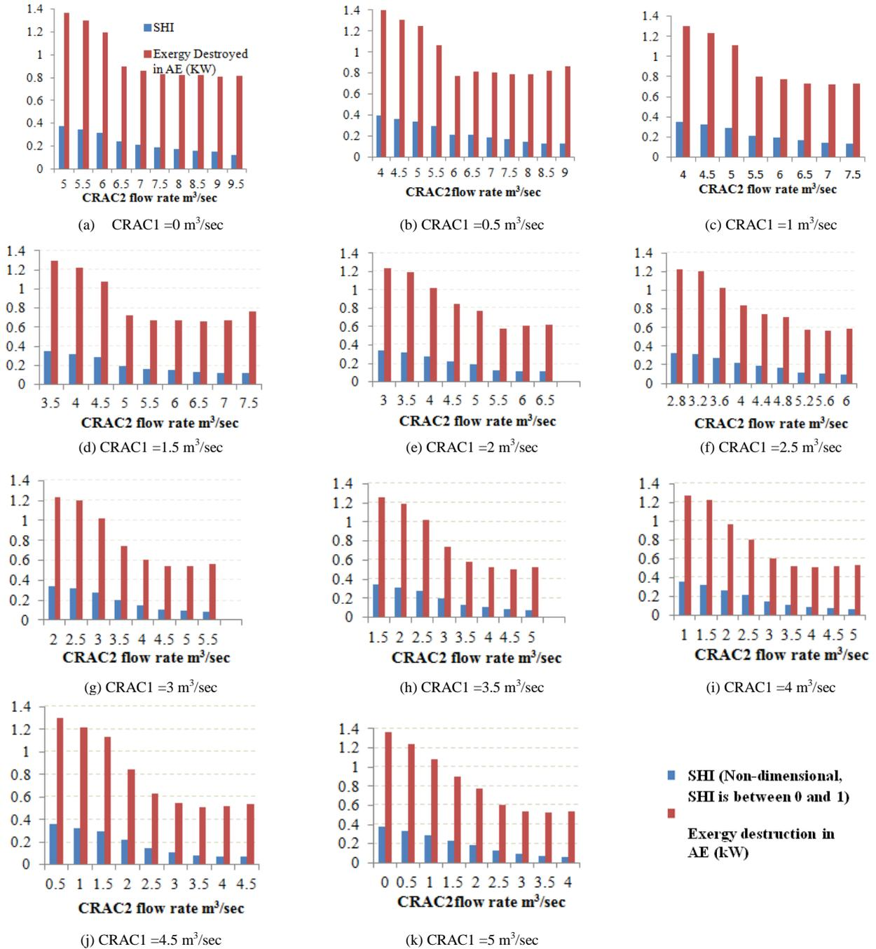
Figure 5. Variation of exergy destruction and SHI at different CRAC flow rates.
