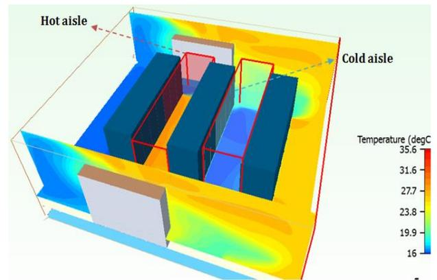
Figure 4. Temperature distribution in a room space.
