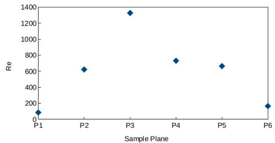
Figure 4: Reynolds numbers through the six sample planes, for the exertion case, with LES model.
