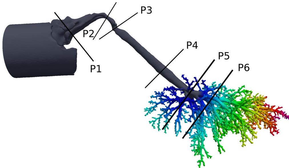
Figure 2: The geometry showing the locations of the sample planes. The geometry is coloured by expansion, with the violet regions indicated maximum expansion and the grey areas, minimum/no expansion.
