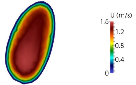
Figure 3: Velocity field through P3, for the exertion case, with a laminar flow solver.
