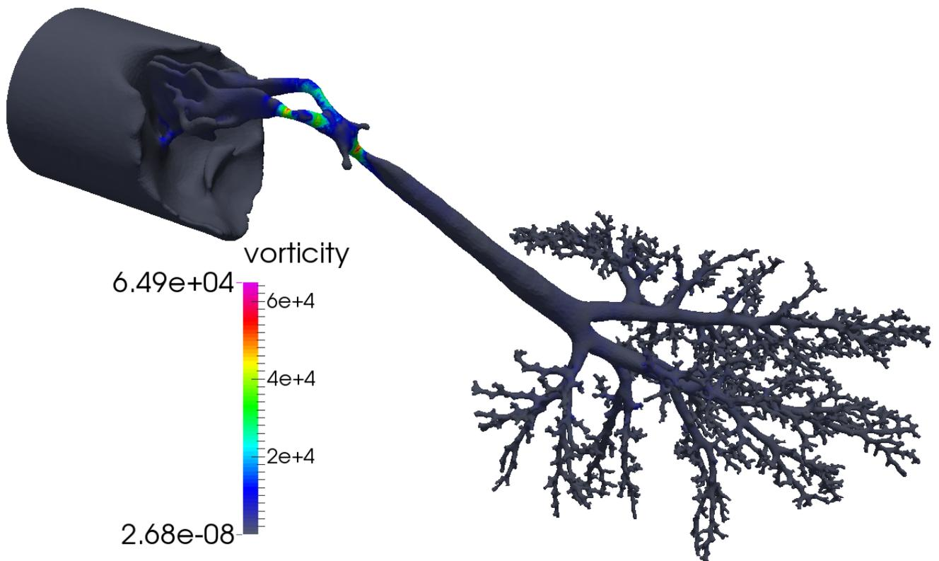
Figure 5: Image of the lung geometry, indicating areas of vorticity. The colour scheme ranges from violet for highest vorticity, to grey for the lowest.
