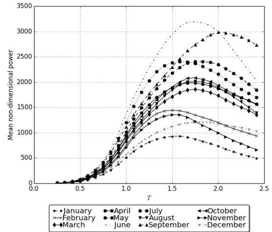
Figure 5: Monthly mean non-dimensional power generated with varying natural period of oscillation and a damping parameter of 0.7
