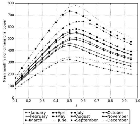
Figure 4: Monthly mean non-dimensional power generated with a varying damping parameter and a non-dimensional natural period of oscillation of 0.83.
