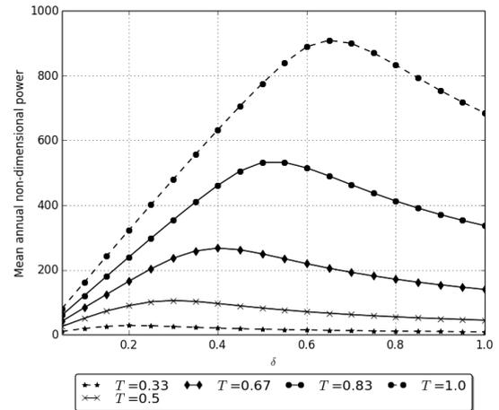
Figure 2: Annual mean non-dimensional power generated for various damping parameters and a non-dimensional natural period of oscillation varying from 0.33 to 1.0.
