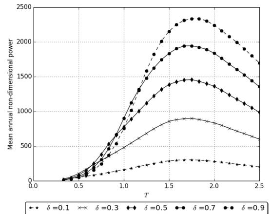
Figure 3: Annual mean non-dimensional power generated for various non-dimensional natural periods of oscillation and damping parameters varying from 0.1 to 0.9.
