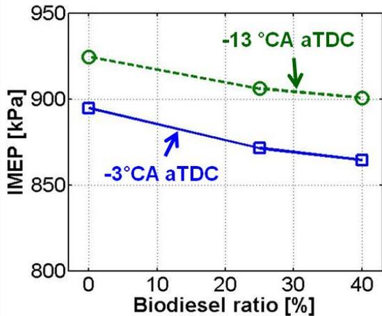
Figure 3. IMEP for three different coconut biodiesel blends and two different injection timings
