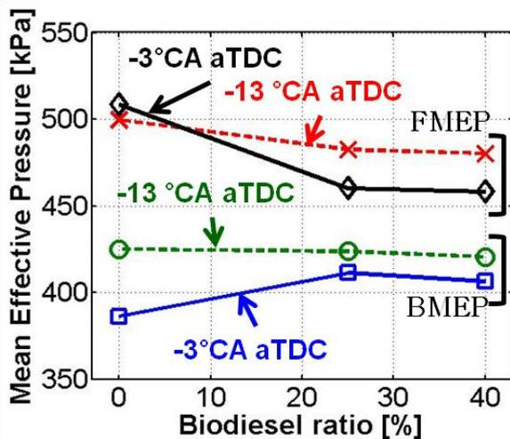
Figure 5. BMEP and FMEP for three different coconut biodiesel blends and two different injection timings
