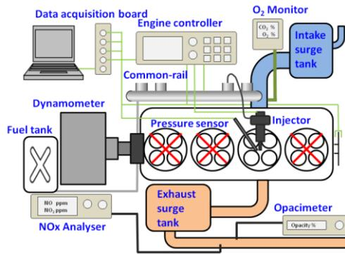
Figure 1. Schematic diagram of single cylinder diesel engine and diagnostic tool.
