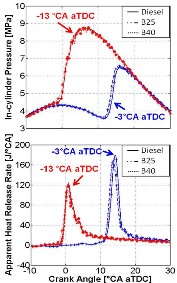
Figure 2. In-cylinder pressure (top) and aHRR (bottom) for three different coconut biodiesel blends and two different injection timings
