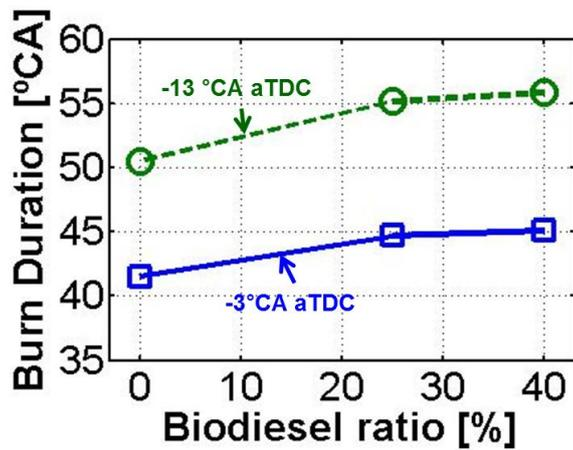
Figure 4. Burn duration for three different coconut biodiesel blends and two different injection timings
