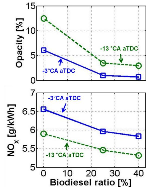
Figure 6. Smoke opacity (top) and NO<sub>x</sub> emissions (bottom) three different coconut biodiesel blends and two different injection timings
