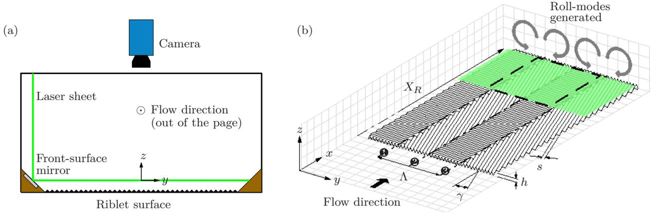
Figure 1. (a) Schematic diagram of the PIV setup showing the cross-section of the wind-tunnel working section; (b) Schematic diagram of the CDA riblets, showing the surface parameters and measurement plane. The circled numbers point out the converging (❶ & ❷) and diverging (❸) regions.
