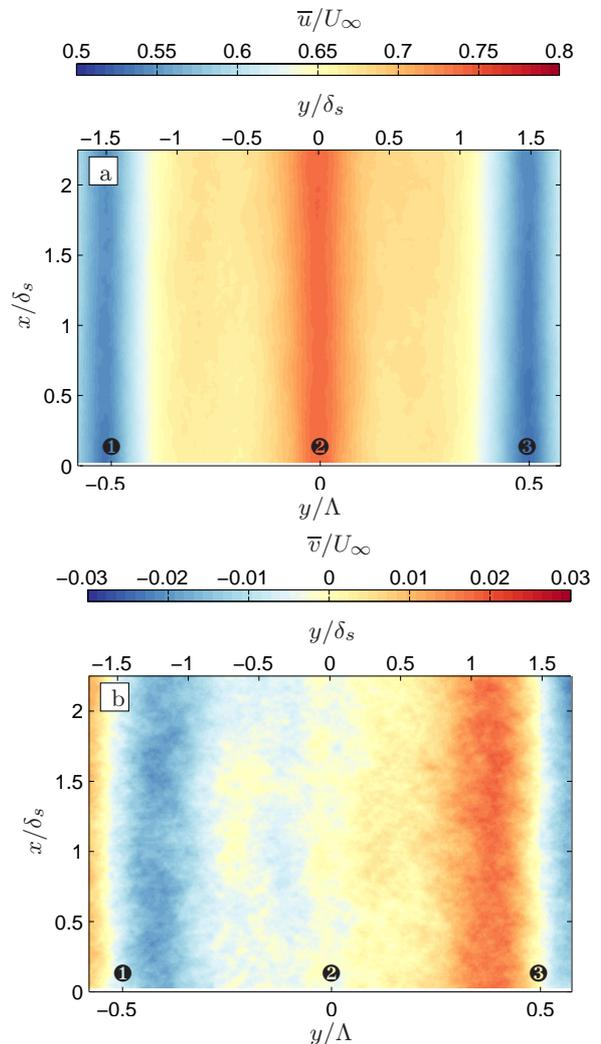
Figure 2. Time-averaged streamwise (a) and spanwise (b) velocity field (normalised by the corresponding freestream velocity  $U_\infty$ ) over the CDA riblets  $z = 5$  mm
