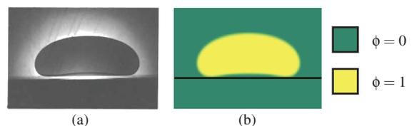
Figure 5. Droplet-scale cross section results for the 0.25 mL case at  $t = 60$  s: (a) experiment [6] and (b) simulation. For illustration, the simulation results have been reflected in the  $rz$ -plane. Image ©1951–1971 AIChE, reproduced with permission.
