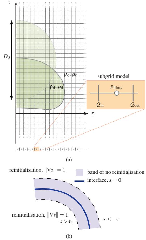
Figure 1. Sketch of modelling approach: (a) droplet-scale domain mesh and subgrid model, (b) level-set reinitialisation scheme.
