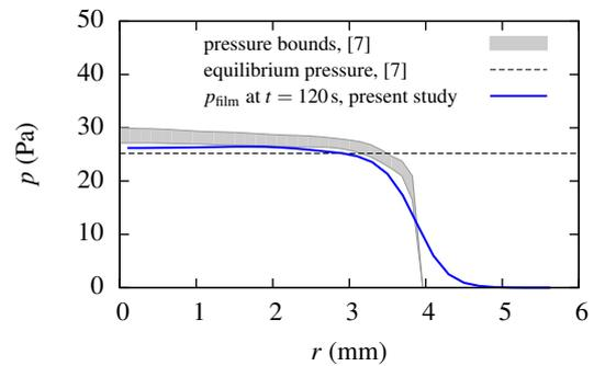
Figure 4. Simulation film pressure,  $p_{\text{film}}$ , and results of Hartland's [7] analysis for the 0.25 mL droplet case.
