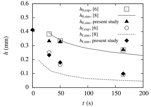
Figure 3. Film thickness at the centreline,  $h_0$ , and at the rim,  $h_f$ , for the 0.1 mL droplet case
