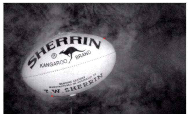
Figure 7: Flow visualisation images of the ball at two orientations. The upper image corresponds to a pitch angle of -90^\circ and the lower image corresponds to 15^\circ pitch, where the red dots indicate the separation points of the boundary layer.
