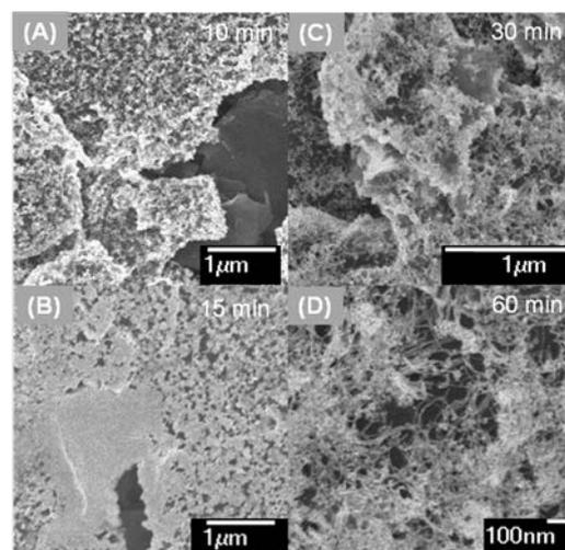
Figure 2. SEM images of gold nanowire on graphite surface with increased surface area, after being immersed in growth solution of (A)10, (B) 15, (C) 30 and (D) 60 minutes.
