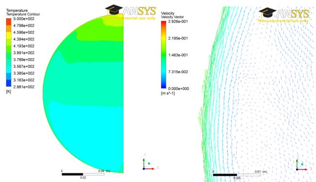
Figure 10. Distribution of (a) temperature ( $T=298\text{--}500\text{K}$ ) and (b) flow velocity ( $V=0\text{--}0.3\text{m/s}$ ) in the tube during preheating [3].
