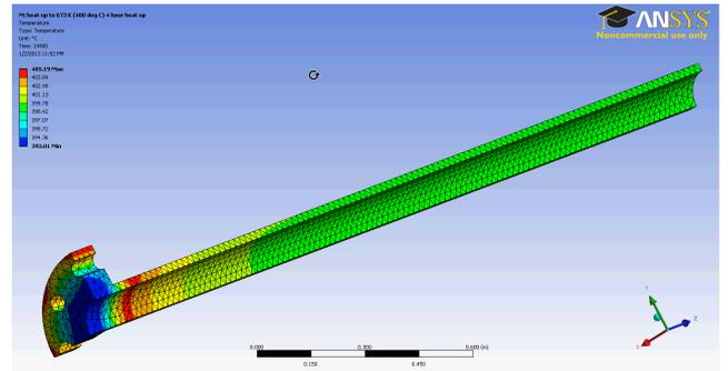
Figure 6. Temperature distribution in a section of the HDT Ludwig tube for preheat to 673K for 3 hours using  $13.9 kW/m^2$  on the flange,  $8.3 kW/m^2$  near the flange and  $3.6 kW/m^2$  on the tube ( $T = 393\text{--}405^\circ C$ ).
