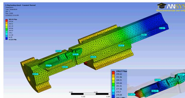
Figure 13. Temperature distribution in the plug valve assembly for a 3-hour, 500K wall preheat ( $T=57-303^{\circ}\text{C}$ ,  $T=166-199^{\circ}\text{C}$ ).
