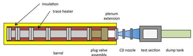
Figure 5. Schematic layout of the HDT showing the heated and insulated Ludwig tube supplying the hypersonic nozzle.
