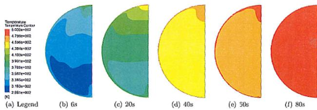
Figure 11. Evolving temperature distributions during the test gas heat up for preheat of 500K and a fill pressure of 50bar ( $T=298-500\text{K}$ ). [3]
