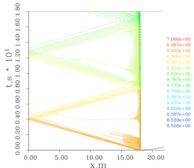
Figure 1. Example x-t diagram of flow in the HDT for fill pressure of 90 bar and preheat of 500K showing the passage of the expansion wave through the Ludwieg tube. (Contours show  $\log(P)$ ).
