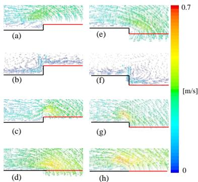
Figure 3. Velocity vectors (coloured by velocity magnitude) in the vicinity of the vibrating plate at different phases of a cycle of vibration. (a) 12.5 % (b) 25 % (c) 37.5 % (d) 50 % (e) 62.5 % (f) 75 % (g) 87.5 % (h) 100%.
