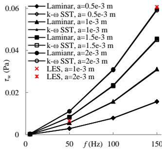
Figure 5. Comparison of the time and space averaged wall shear stress.
