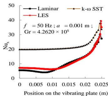
Figure 6. Time averaged profile of local Nusselt number over the vibrating heated plate.
