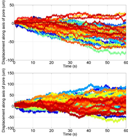
Figure 5. Displacement of a single particle along the axis of the drift ratchet pore illustrated in figure 2, using the model developed in this paper, for 50 separate particles. (Top) Case 1 and (Bottom) Case 2. The conditions of the simulation are as shown in table 2. The direction of displacement coincides with the orientation of the pore profile in figure 2. Initial position of all particles is at the origin.
