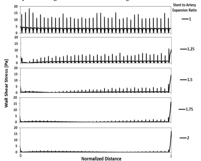
Figure 3. Comparison of the distribution of the wall shear stress on a line in the axial direction of the artery within the stented region for all five stent-to-artery deployment ratios
