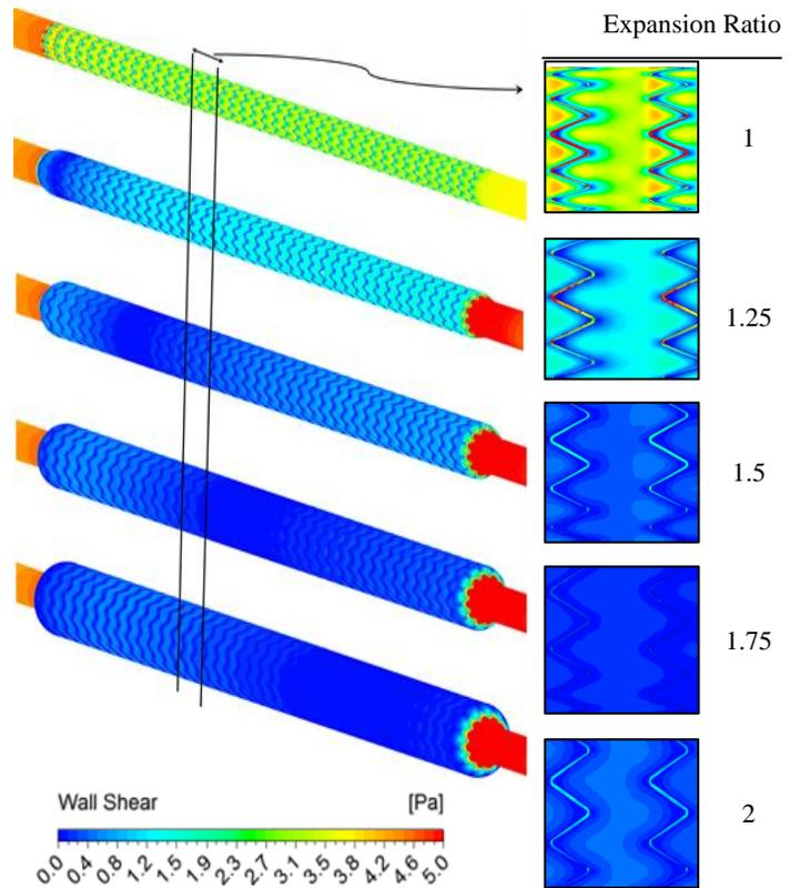
Figure 2. Wall shear stress distribution within the stented portion of five arteries with different sizes of stent-to-artery deployment ratios. The blood flow direction is from left to right.
