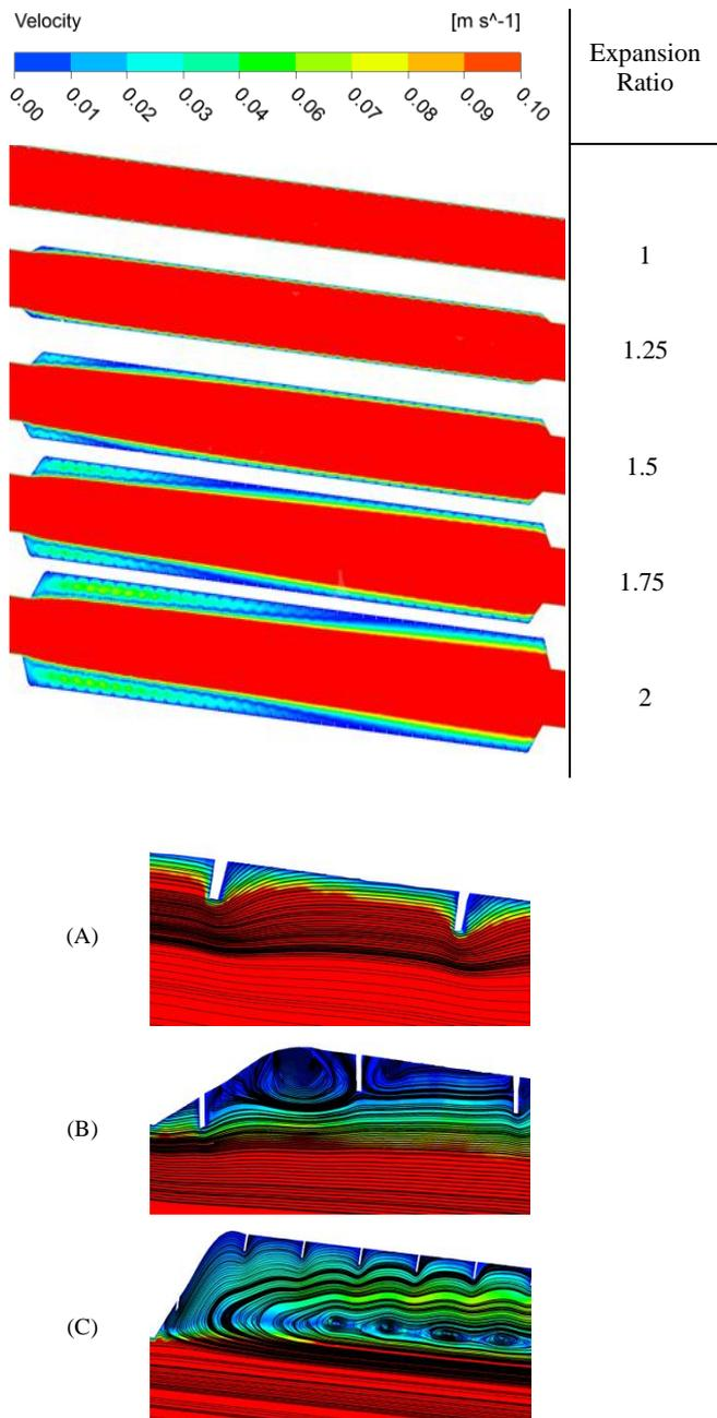
Figure 4. Velocity contour plots projected on the mid-longitudinal plane for five different configurations of the stented artery made with regard to various stent-to-artery expansion ratios.
