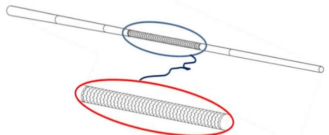
Figure 1. Schematic view of the stented femoral artery divided into three sections with stent placed at the middle section.
