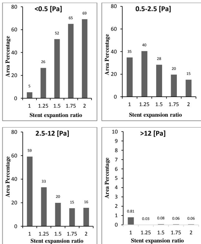
Figure 5. Percentage of the vessel wall area exposed to low (<0.5 Pa), moderate (between 0.5 and 2.5 Pa), high (between 2.5 and 12 Pa) and greater than 12 Pa (induces platelet aggregation) WSS for all five stent-to-artery expansion ratios.
