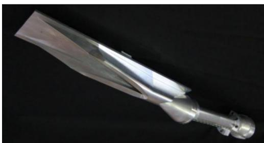
Figure 1: Mach 12 REST scramjet test article
