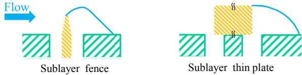
Figure 7. Separating streamline expected for the rectangular plate and fence with edge.
