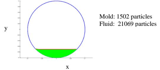
Figure 1. detection of boundary particle for a cylinder mold rotating around its main axis. The mold is shown in blue, the inner particle in green and boundary particle in red colour.
