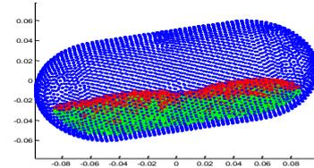
Figure 2. Detection of boundary particle in three dimensional configurations. The mold is shown in blue, the inner particle in green and boundary particle in red colour.
