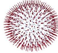
Figure 4. Particle position of 3D sphere (radius=0.1m) with the normal vector on the surface.
