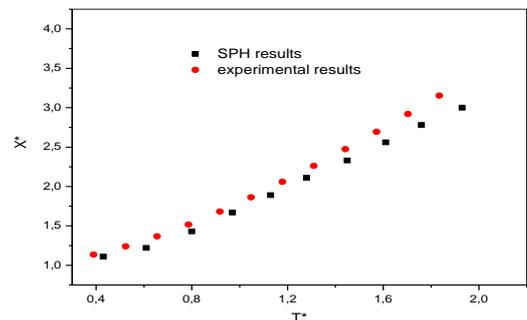
Figure 5. Surge front for experiment (●) and SPH simulation (■).
