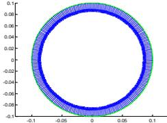
Figure 3. Particle position of 2D circle (radius=0.1m) with the normal vector on the surface.
