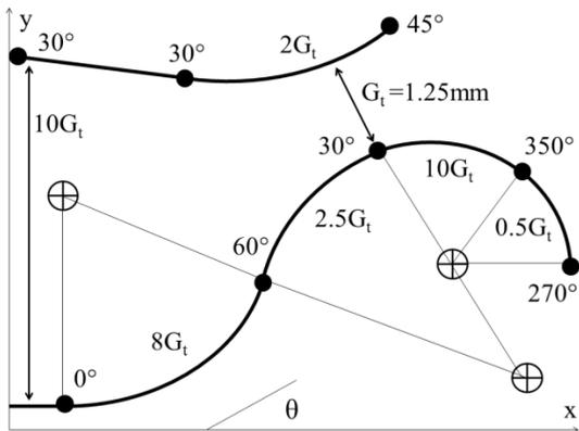
Figure 2. Flow deflector geometry
