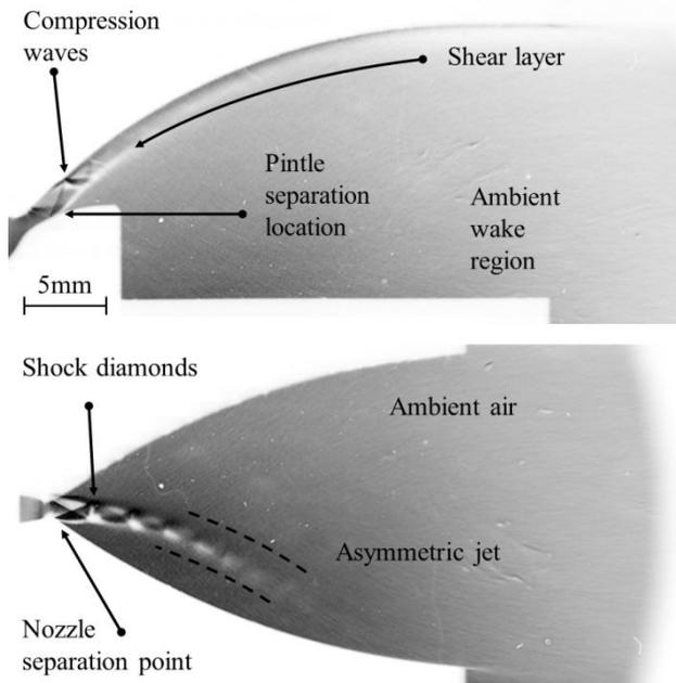
Figure 5. ED and CD flow structure at PR ~ 5
