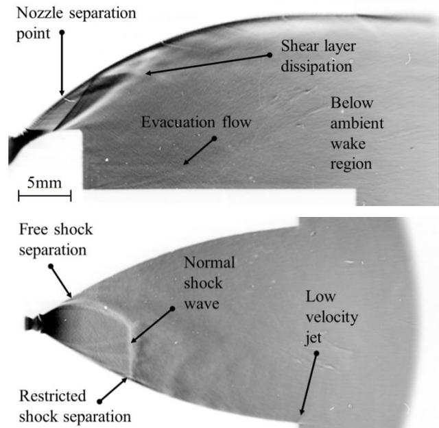
Figure 7. ED and CD flow structure at PR ~ 15
