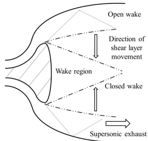
Figure 1. Flow features in the ED nozzle
