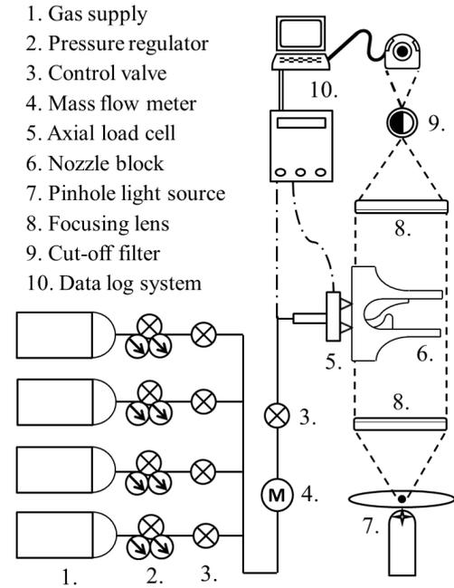
Figure 3. Diagram of experimental setup
