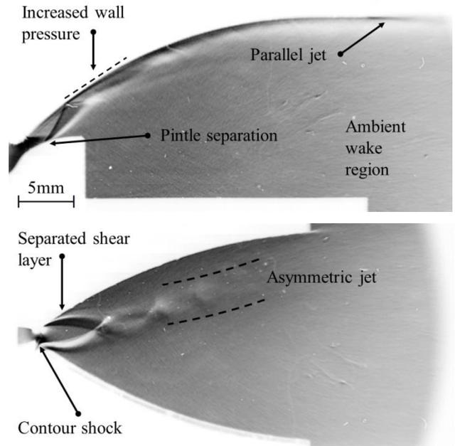
Figure 6. ED and CD flow structure at PR ~ 10
