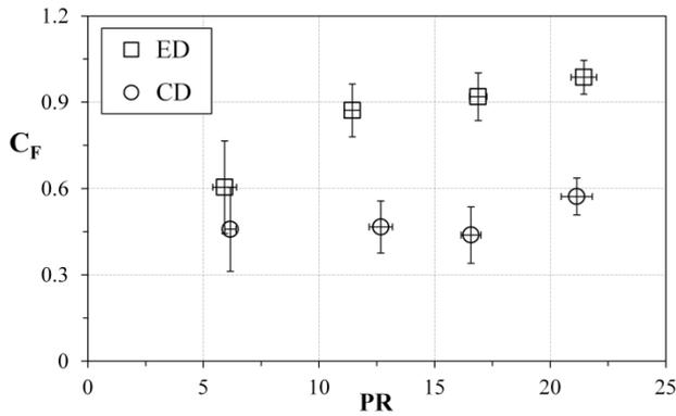
Figure 4. Comparison of nozzle thrust coefficient for individual tests
