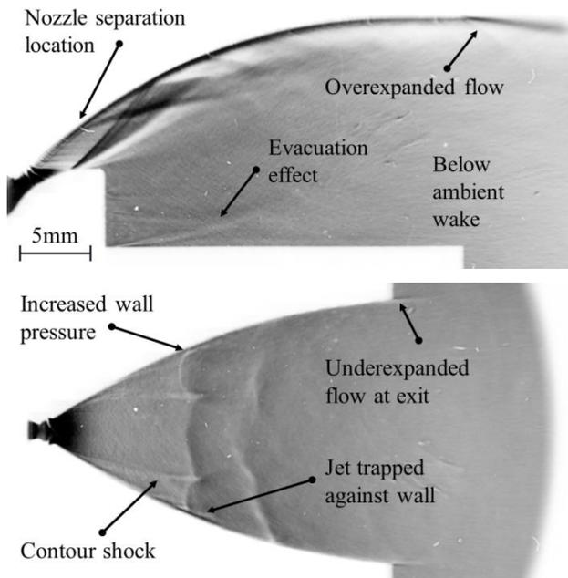
Figure 8. ED and CD flow structure at PR ~ 20
