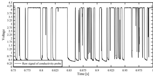
Figure 3. Raw Voltage signal of a phase detection conductivity probe ( $\varnothing = 0.25$  mm):  $d_w/h = 1.28$ ;  $q_w = 0.143$  m<sup>3</sup>/s;  $Re = 5.7 \times 10^5$
