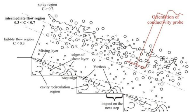
Figure 2. Sketch of stepped spillway skimming flows and positioning of phase-detection probe in the intermediate flow region for  $0.49 < C < 0.51$
