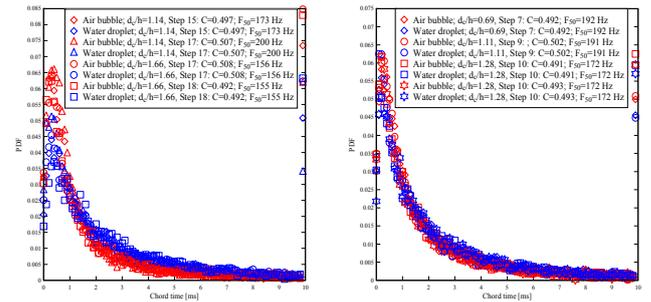
(A) Chord times for  $150 \text{ Hz} < F_{50} < 200 \text{ Hz}$ ;  $h = 0.05$  cm
