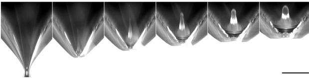
Figure 4: Evolution of internal jet formed as a bubble detaches from a 2.5 mm radius orifice over six consecutive images with 200  $\mu\text{s}$  between images. The black bar in the bottom right corner represents 1 mm.
