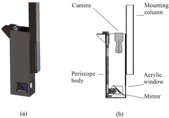
Figure 1. Carriage mounted periscope (a) 3D view (b) Section view
