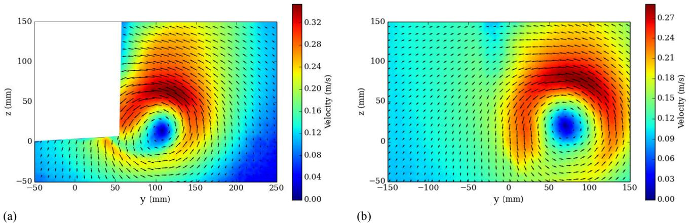
Figure 6. 2D velocity vectors plots averaged over 128 double frames on an 8 x 8 grid for (a) Plane 1 (b) Plane 2
