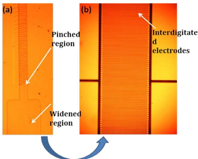
Figure 1. Overview of DEP-active hydrophoretic device. (a) PDMS micro-channel consisting of pinched and widened channel. The slight difference of particle trajectories can be expanded after entering the widened channel. (b) Interdigitated electrodes were patterned onto the bottom of the channel which generated a negative DEP force to push particles upwards.
