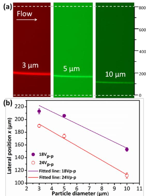
Figure 2. Calibration of the microfluidic device for DEP-active hydrophoretic sizing. (a) Optical microscopy images showing position distributions of 3, 5, 10  $\mu\text{m}$  beads in the widened channel. (b) Lateral positions of particles as a function of their diameters. The solid lines were linear regression lines to obtain calibration lines for particle sizing at 18 and 24  $V_{p-p}$ , respectively. The average experimental value of lateral positions was measured 3 times.
