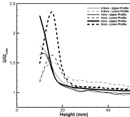
Figure 4. Comparison of the upper and lower velocity profiles between foamed cylinders with 40mm thickness at 75°C
