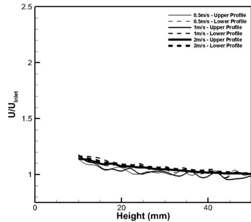
Figure 5. Comparison of the upper and lower velocity profiles between foamed cylinders with 10mm thickness at ambient temperature
