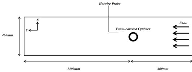
Figure 1. Side view of experimental setup
