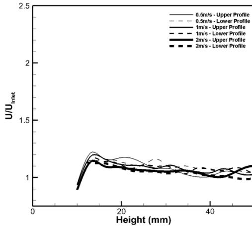
Figure 3. Comparison of the upper and lower velocity profiles between foamed cylinders with 40mm thickness at ambient temperature
