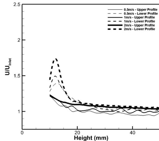
Figure 6. Comparison of the upper and lower velocity profiles between foamed cylinders with 10mm thickness at 75°C
