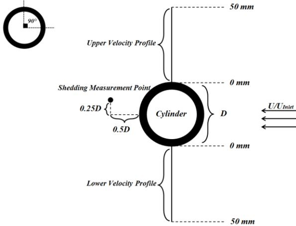
Figure 2. Schematic of hotwire measurements
