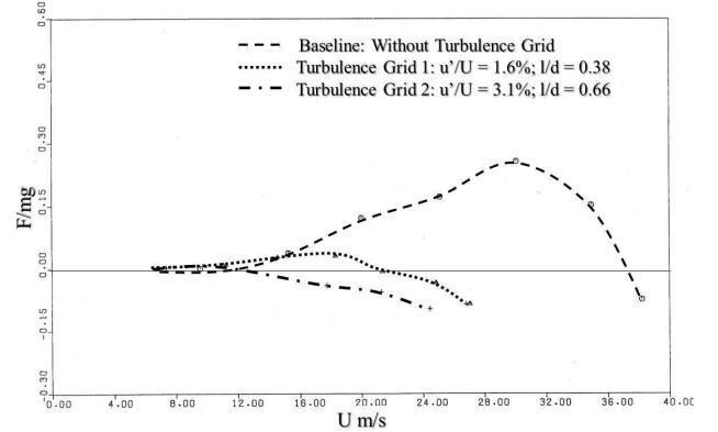
Figure 8. Effects of free-stream turbulence on cricket ball swing. New 4-piece ball, seam angle =  $20^\circ$ , spin rate = 5 revs/s.
