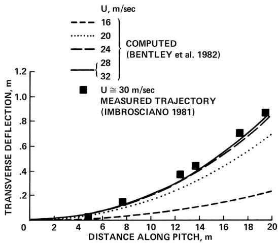
Figure 5. Comparison of computed flight paths using measured forces for the cricket ball with the best swing properties. Seam angle =  $20^\circ$ , spin rate =  $14 \text{ revs/s}$ .
