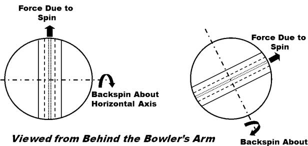
Figure 12. Schematic for spin-induced “Malinga” swing.
