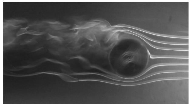
Figure 10. Dye flow visualization over a spinning cricket ball in a water channel. Flow is from right to left and the ball is rotating in a clockwise direction.
