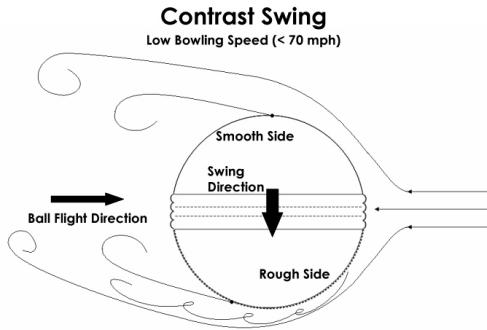
Figure 9a. Schematic for flow over a ball for contrast swing at relatively low bowling speeds.
