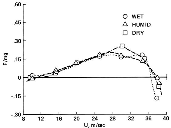
Figure 15. Effect of humidity on the measured side forces on a spinning cricket ball. Seam angle = 20°, spin rate = 5 revs/s.
