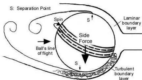
Figure 1. Schematic of flow over a cricket ball for conventional swing.
