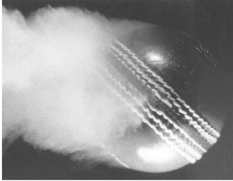
Figure 2. Smoke flow visualization of flow over a cricket ball. Flow is from right to left. Seam angle = 40°, flow speed = 17 m/s,  $Re = 850,000$ .
