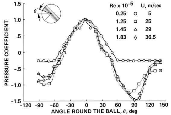
Figure 3. Pressure distributions on a cricket ball held at a seam angle of 20°.
