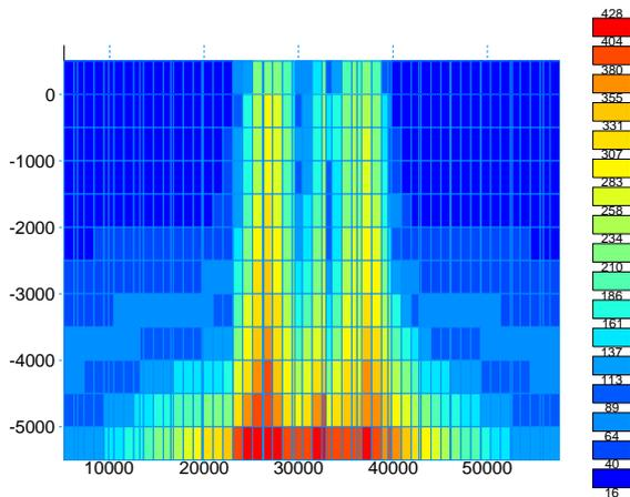
Figure 4: A NW-SE vertical temperature section, bearing 150° north, showing the Wairakei (left) and Tauhara (right) plumes from Model 4.6c. The scale bar units are in °C.
