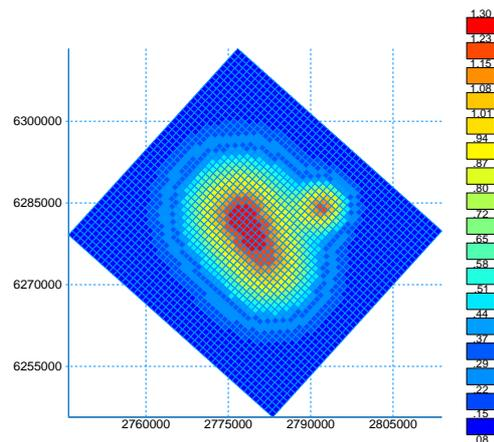
Figure 3: Non-uniform heat input for Model 4.6. The scale bar units are  $\text{W/m}^2$ .
