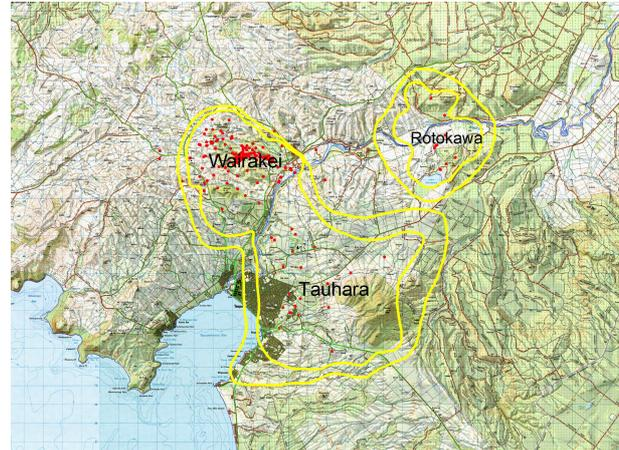
Figure 1: Wairakei, Tauhara and Rotokawa geothermal field locations. The lake at the left is Lake Taupo, and the Waikato River runs up to the north-east. The yellow band shows the resistivity boundaries
