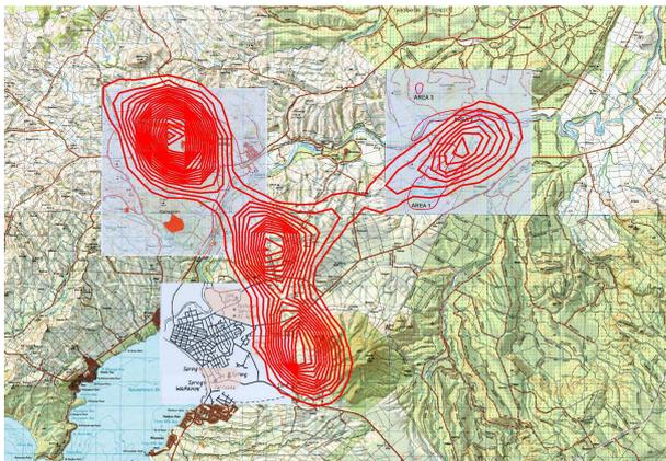
Figure 5: Surface heat flow contours from Model 4.6c including cap rock
