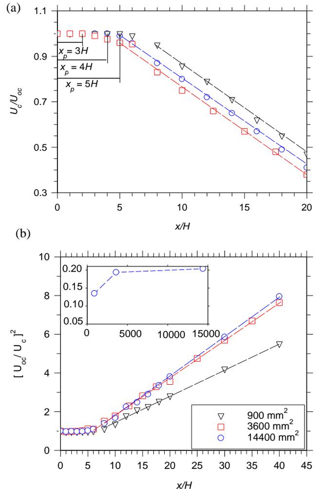
Figure 1: The normalized mean velocity decay (a) in the near field (b) in the far field.
