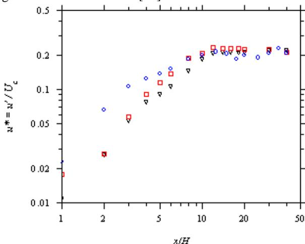
Figure 2: The centerline turbulence intensity field for the three cases. The definitions of the symbols are identical to those in Figure 1.
