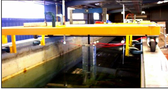
Figure 3. Wave flume with cylinder attached to the fixed carriage [7]
