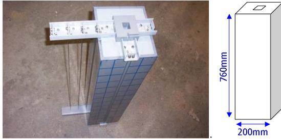
Figure 2. Cylinder model with probes attached [7]
