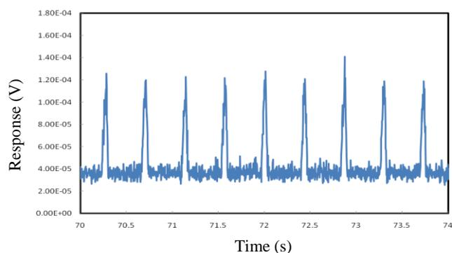
Figure 4. Signal of droplets passing through the red laser detection zone.
