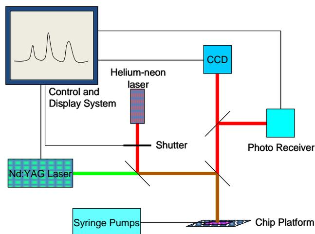
Figure 2. Schematic of microPIV system set-up.
