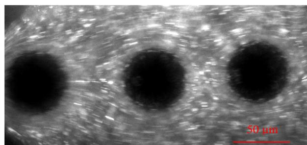
Figure 3. CCD image of the droplets generated at a liquid flow rate of 1  $\mu$ L/h and an oil flow rate of 10  $\mu$ L/h.
