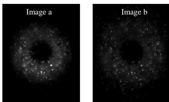
Figure 5. The double PIV images of droplet-forming flow.
