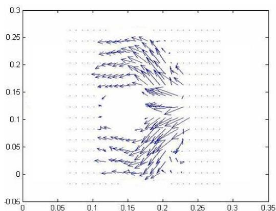
Figure 6. The computational velocity field from one set of double images.
