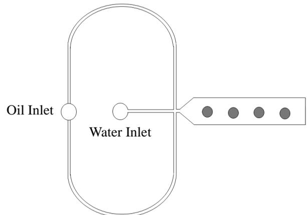
Figure 1. Schematic of co-flow focusing droplet generation chip. All channels are 70  $\mu\text{m}$  deep and 50  $\mu\text{m}$  wide, except the droplet collection channel which is 200  $\mu\text{m}$  wide.
