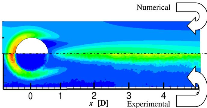
Figure 6. Temperature contours obtained using both numerical and experimental data for  $Re = 568$ .
