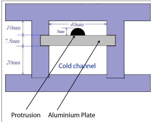
Figure 2. A cross-section through the channels of the heat exchanger, showing the location of the protrusion in the warm water channel.
