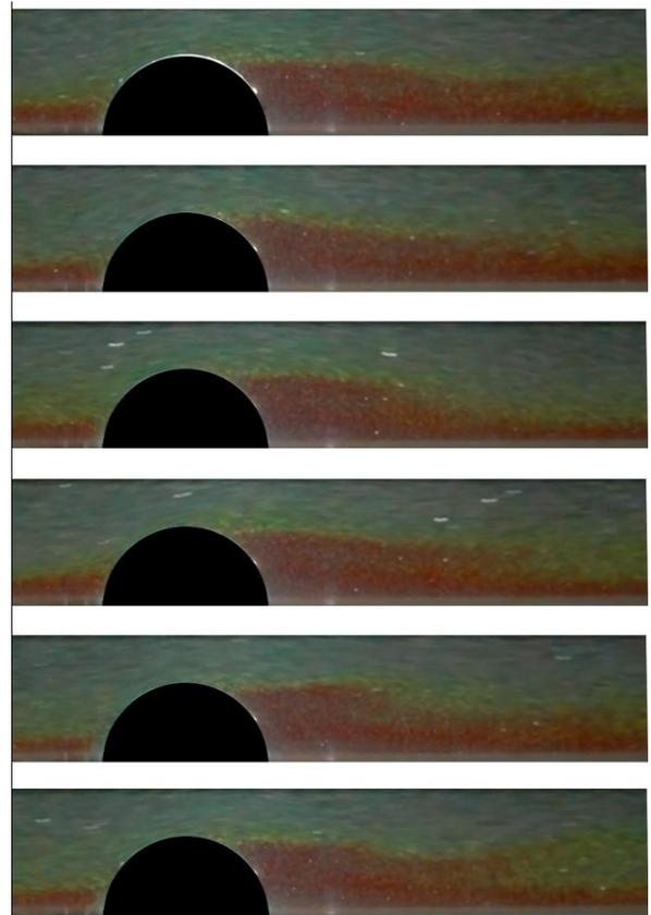
Figure 5. A 2s sequence of raw images from the in-plane TLC experiment showing unsteady behaviour in the wake of the protrusion.
