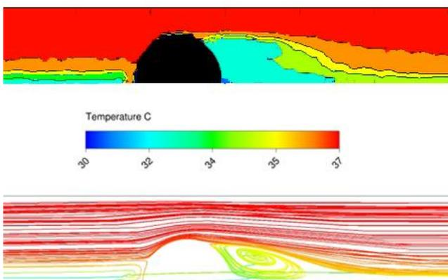
Figure 4. (top) Post-processed TLC and (bottom) CFD pathlines coloured by temperature indicate the extent of mixing,  $Re = 1025$ .
