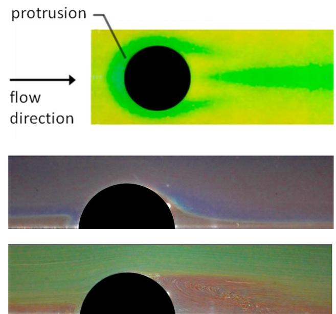
Figure 3. Typical image obtained from the experiment: (top) the sheet during a calibration test, and (below) in-plane, with colour enhancement, for  $Re$  of approx 550 and (bottom) 1025.
