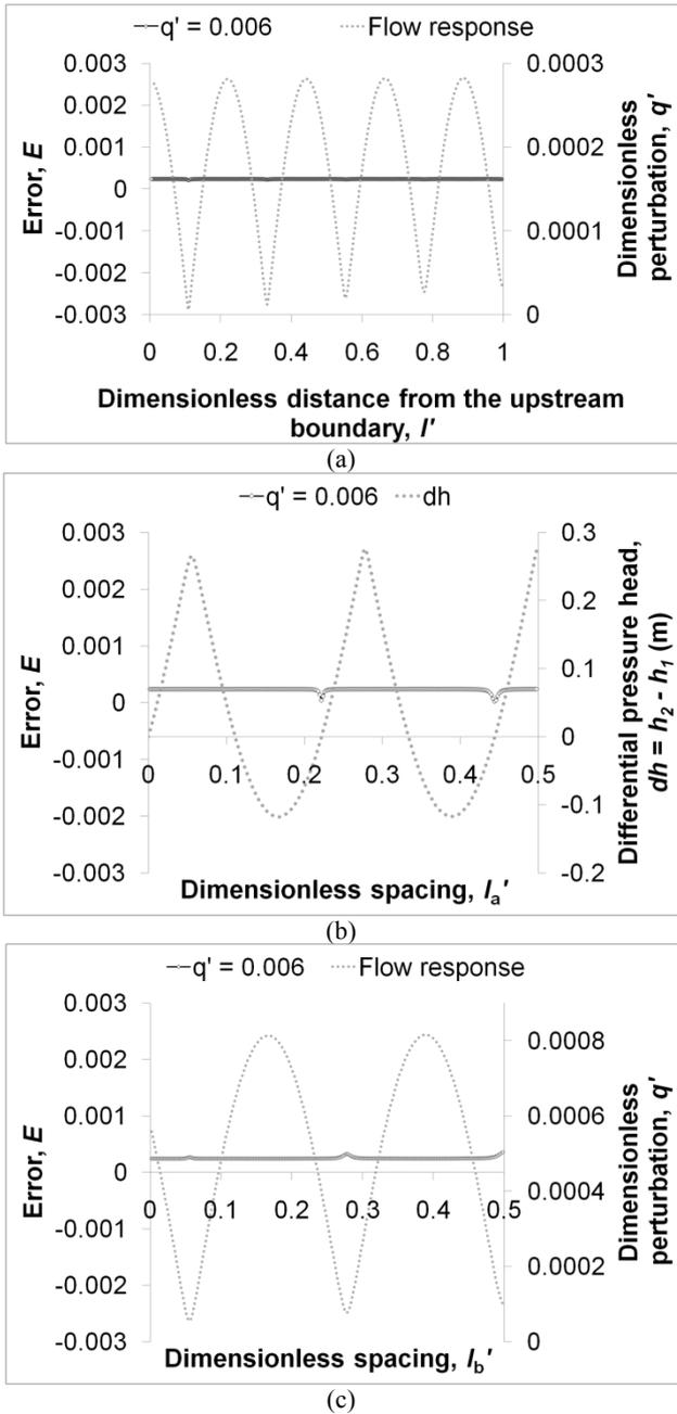
Figure 5. Effect of the configuration of the KDP unit on the error: (a) magnitude error in the case in figure 4 (a), (b) magnitude error in the case in figure 4 (b), (c) magnitude error in the case in figure 4 (c)
