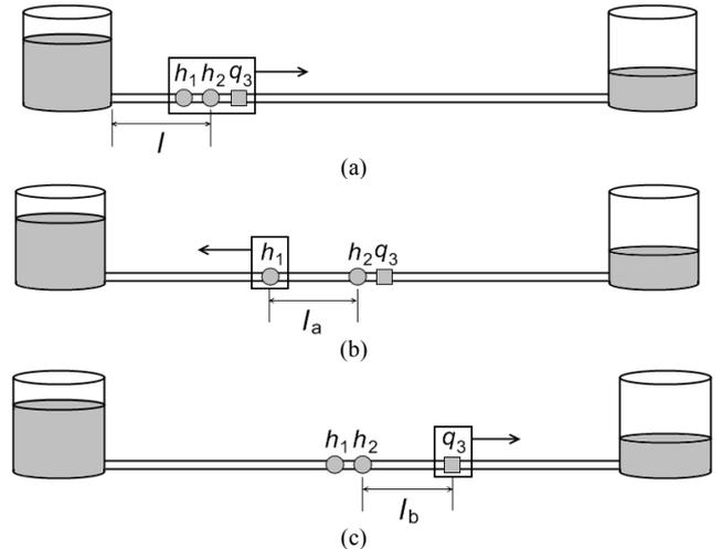
Figure 4. KDP configurations investigated in the analysis, showing the distances involved in each scenario
