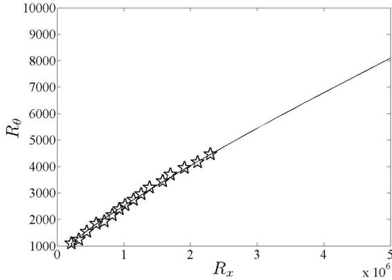
Figure 5: Evolution of momentum thickness Reynolds number ( $R_0$ ) for different streamwise Reynolds number ( $R_x$ ). Star ( $\star$ ) symbols represent the experimental data points, the solid line corresponds to evolution calculations with same initial conditions as the experimental data.
