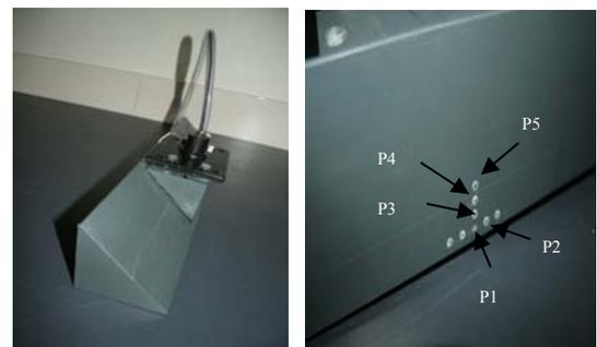
Figure 4: Photo graph showing (a) the wedge at 5° angle (with insertion block) and (b) pressure sensors position
