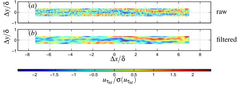
Figure 2: Example velocity signals from the spanwise array (a) unfiltered raw data; (b) 2-D Gaussian filter of size  $0.5\delta \times 0.16\delta$  (streamwise, spanwise) applied. Colour shows fluctuating skin friction velocity normalised by the standard deviation. Signals are projected in  $x$  using Taylor's Hypothesis and a convection velocity of  $U_c^+ = 20$ .
