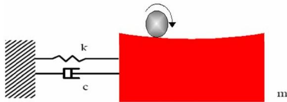
Figure 1. Proposed design with the cylindrical absorber for a structure of mass  $m$ , stiffness  $k$  and coefficient of damping  $c$ . When the structure experience a horizontal displacement, it causes the cylinder to roll on the ramp, while the granular flow of the particles inside dissipates the energy.
