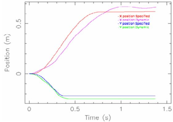
Figure 5. Histories of the container x and y position for the specified and dynamic motion cases.
