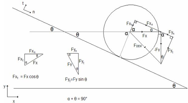
Figure 3. Diagram of the rolling cylinder, ramp and the relevant forces. Global coordinates are  $x, y$ . Local coordinates are  $n, t$ .
