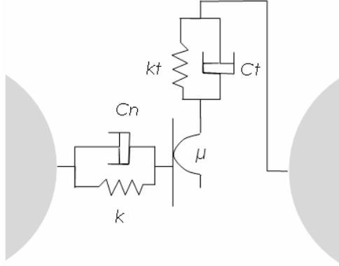
Figure 2. Schematic representation of DEM model.
