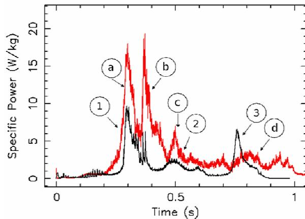
Figure 8. History of the input power to the system due to the particle torque on the container boundary for the dynamic case (red) and the specified case (black).
