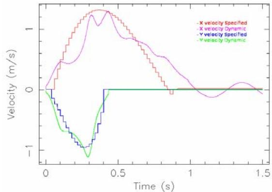
Figure 6. Histories of the container x and y velocity for the specified and dynamic motion cases.
