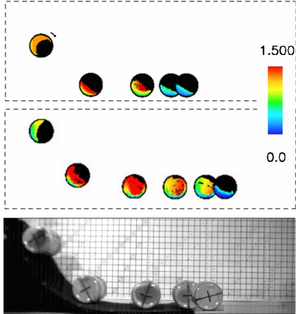
Figure 4. Motion of cylinder down ramp for specified case (top), dynamic model (middle) and for experiment (bottom).
