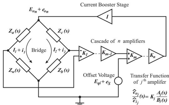
Figure 1: Model of constant-temperature hot-wire anemometer. From Watmuff [11].
