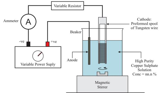
Figure 2: Schematic of apparatus for copper plating of spool of tungsten wire.
