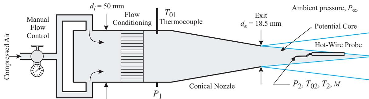
Figure 3: Schematic of apparatus constructed for calibration of hot-wire probes at high-speeds.
