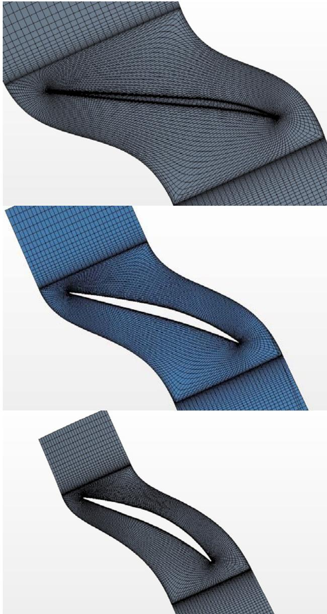
**Figure 2 – Details of hub (bottom), blade-to-blade mid span (mid) and shroud (top) computational grids**
