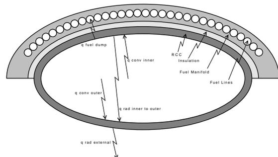
Figure 1: Combustor cross-section
